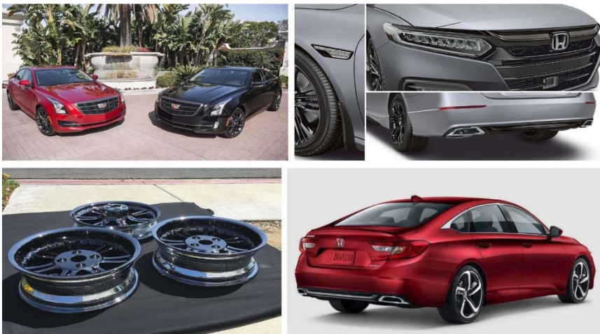
Figure 6 - Examples of black chromium finishes for automotive applications: (Clockwise from upper left) Cadillac black chromium finish on CTS and ATS models; Honda Accord black chromium grille accent; Honda Accord rear garnish; automotive wheel rims.
