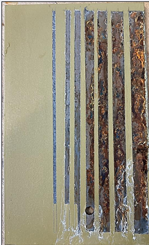
Legacy coating after 26 hours of salt spray exposure.
