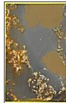
CH1050: After 1050°F/1000 hrs & after 24 hrs of salt spray exposure
