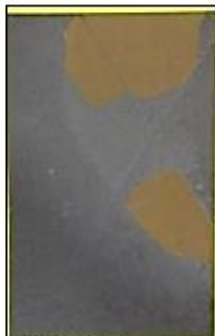
CH1050: After 1050°F/1000 hrs & before salt spray exposure
