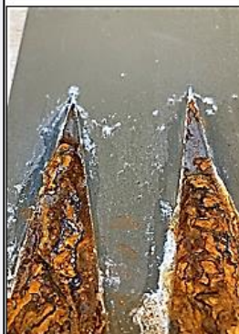
Close up of left apexes of Q42 after 72 hrs of exposure
