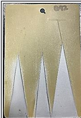
Q42 prior to throwing power testing. The gray triangle is the area of removed coating.
