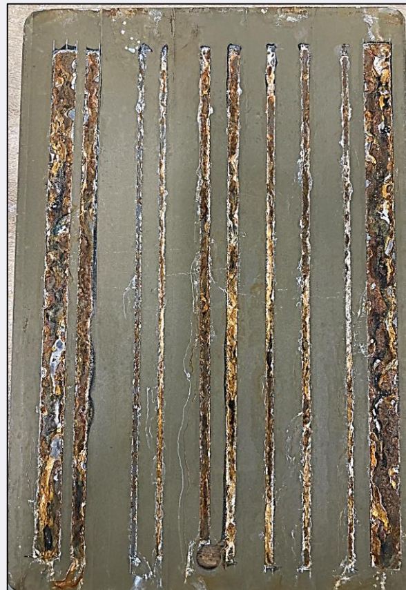
Aseal 5KGT after 26 hours of salt spray exposure.
