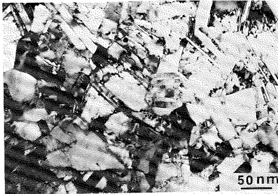
Fig. 6—TEM micrograph of as-plated Pd electrodeposit.
