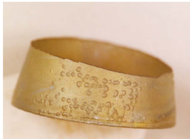
Figure 3 - Formation of blisters on zinc plated parts, subjected to embrittlement relief heat treatment around 230°C for 24 hours.
