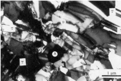
**Figure 17** - Transmission electron micrograph of a nickel electrodeposit.
